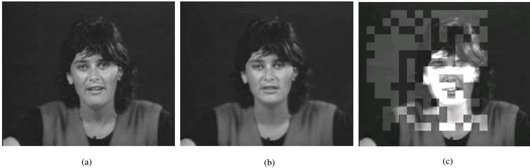
Figure (5.11): Samples of Miss America video frames. (a) Current frame. (b) Previous frame. (c) The difference blocks between current and previous frame using Three-step technique.
